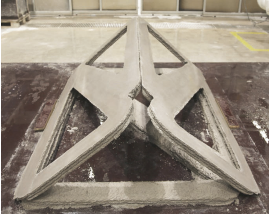
Fig. 2 Assembled prototype element demonstrating proof of concept for a project at Technische Universität Braunschweig. (Image courtesy of Norman Hack)
