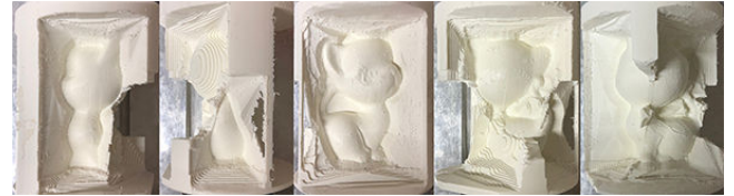
Figure 16: Finishing phase. Side regions finished with a 1mm ball cutter.
