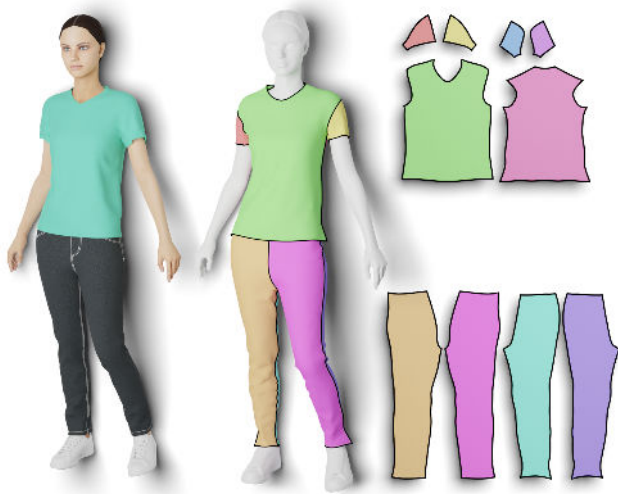
Fig. 23. Our method computes sewing patterns (right) for the input meshes of a shirt and pants (left). To validate our result, we virtually sew our resulting patterns and then drape them using the physically based simulation of CLO [CLO 2022] (center).
