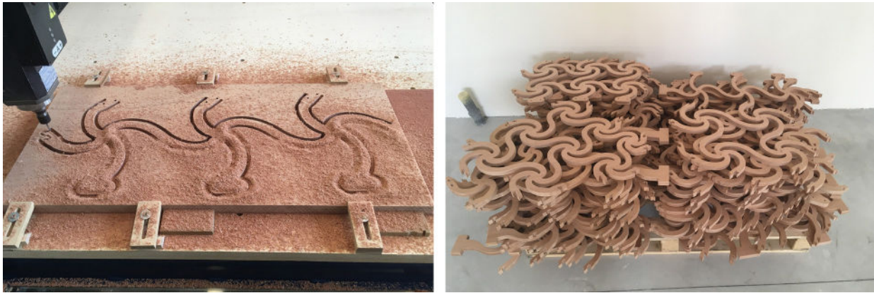
Figure 14: Fabrication of the FlexMaps patches
