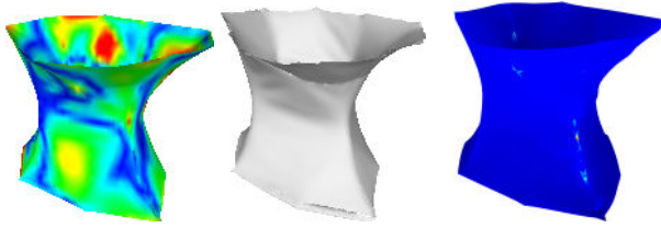
Fig. 10. Visualization of the Hausdorff distance between our tensile structure (left) and the physical replica (center). Red indicates a deviation of 2% relative to the bounding box diagonal. Right: Thin shell simulation of a thick fabric ( t = 1.2 mm, E = 120 MPa, \nu = 0.35 , \rho = 250 kg/m 3 ), yielding a maximum strain of 10.6% and an average strain of 0.18%.
