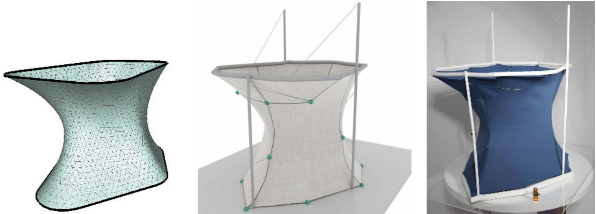
Fig. 1. We present a novel method for approximating input models (left) with tensile-like surfaces. Our method automatically decomposes the target mesh into near-developable patches, identifies a sparse set of supports, and generates a sparse set of tension strings (middle). The output of our method captures the high visual appeal of tensile structures and is ready for fabrication (right).
