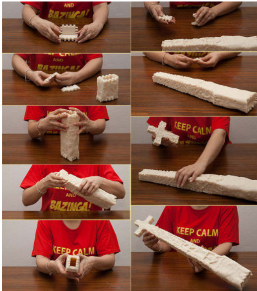
Figure 17: The approach proposed in [ACP*14] breaks down the original shape into a set of height fields that can be individually manufactured without requiring support material and can be assembled manually to build a self-supporting structure.
