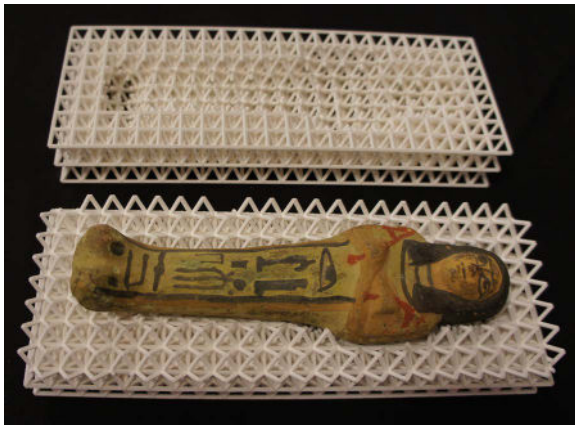
Figure 10: An example of a wire-frame lattice structure designed and produced to tightly fit around the shape of the artwork, for packaging and transport.
