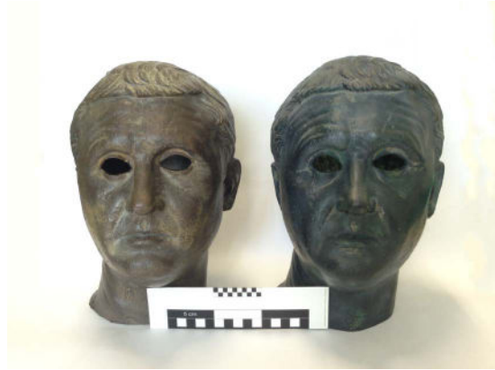
Figure 5: Hand painting and accurate finishing can significantly improve the final appearance of a fabricated replica (head of the Arringatore statue, Archaeological Museum, Florence). The head on the right is in white resin printed by a photopolymerization technique and painted to look like ancient bronze; the one on the left is actually in bronze. Note that the original patina of the Arringatore statue is more similar in color to the painted replica version than the new, bright bronze replica.
