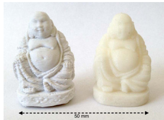
Figure 3: Two small buddhas fabricated in ABS using two different FDM machines. Given the limited size of the objects, the layer structure is quite evident. Note that, depending on the appearance properties of the material, the small scale details and the printing artefacts can be evident to a greater or a lesser extent.
