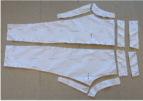
Figure 24: The fabrication process of a pair of leggings. The printed patterns are equipped with extra space (seam allowance) to facilitate sewing. We also place labels to guide the sewing process.
