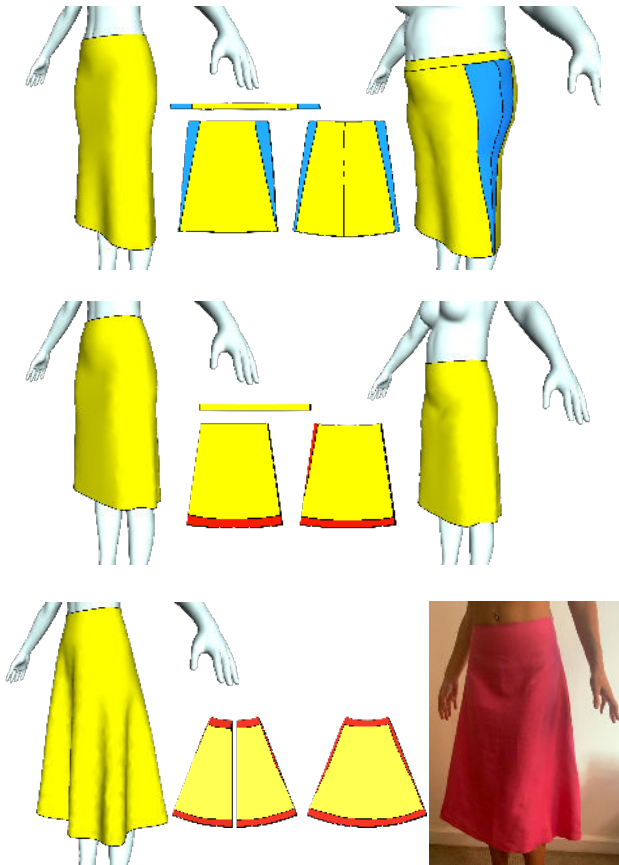
Figure 22: Different adaptations of loose skirts and final fabrication. Left: the reference fit; right: the altered version.
