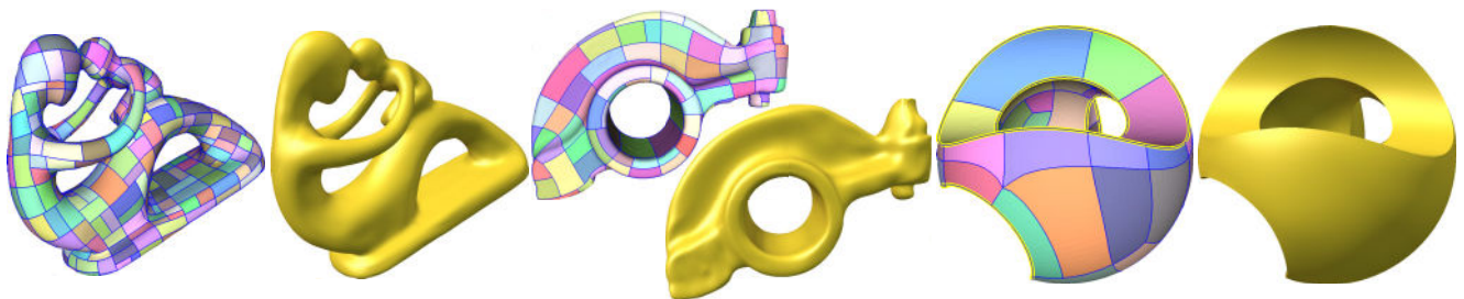
Figure 19: Several T-spline models obtained by least-squares fitting from T-meshes generated by our algorithm: fertility, rockerarm, sculpt.
