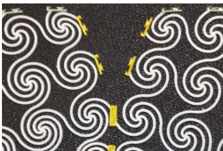
Fig. 13. A closeup of the connectors used to secure FlexMaps across seams.
