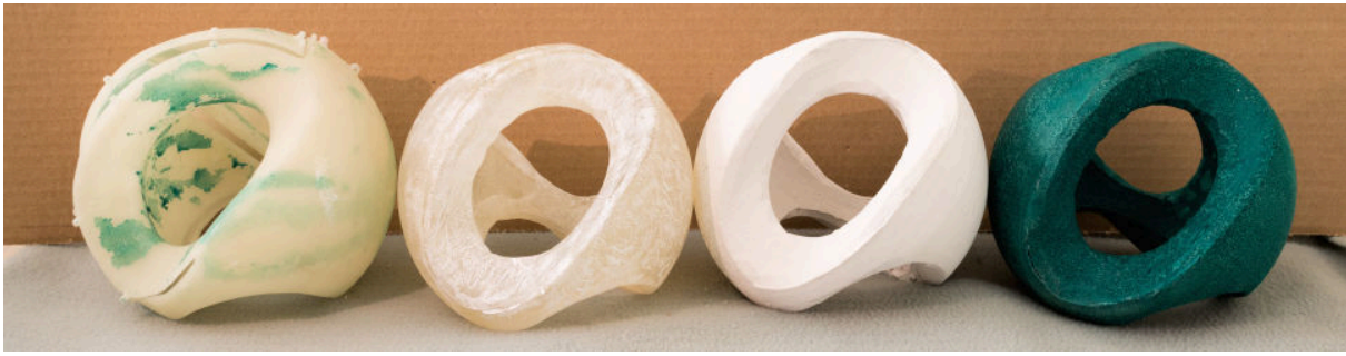
Figure 6: Sculpt model. Left to right: the flexible mold, the result of the cast using neutral resin, the cast with gypsum, and the cast with colored resin.
