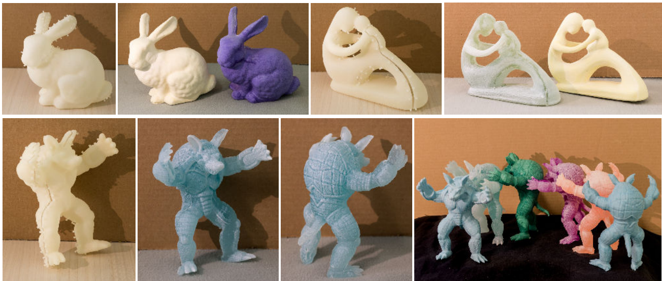
Figure 22: Molds and casts obtained for the bunny, the fertility, and the armadillo models.
