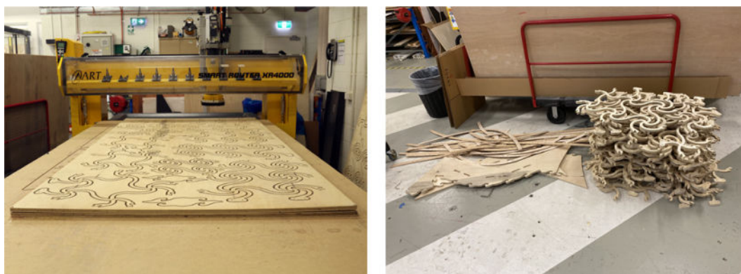
Fig. 18. Fabrication of the demonstrator: CNC cutting and components after sanding.
