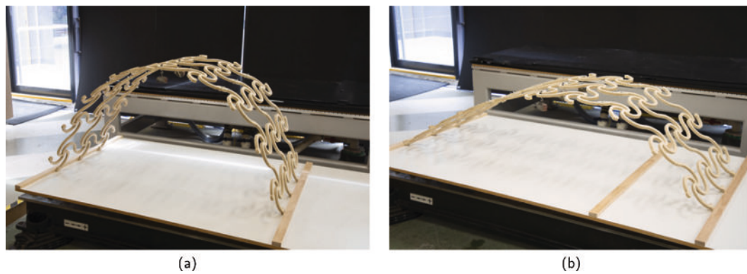
Fig. 8. Experimental test on a three-panels arch made of all equal spirals, the structure is loaded on the three spirals of the mid section with 0.5, 1.0 and 1.5 kg: (a) first setup with a span of 1.5 m; (b) second setup with a span of 2.0 m.
