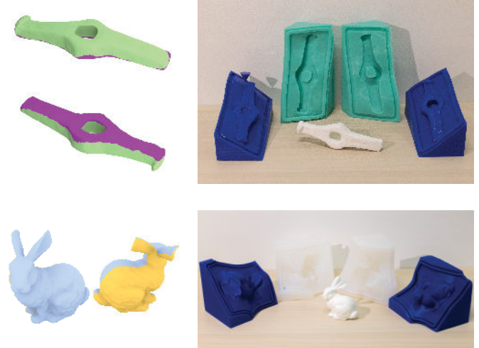
Fig. 15. Some simple models cast with our technique. Left: the optimized segmentation; right: the fabricated metamolds and the cast object.
