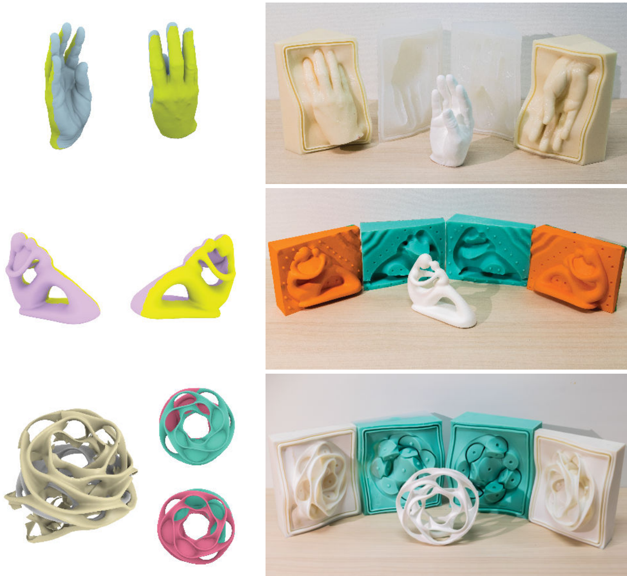
Fig. 19. Successful casting of objects which could not be fabricated with the approach in [Herholz et al. 2015]. The heptoroid (third row) is a failure case also for FlexMolds [Malomo et al. 2016], which derives an extremely complex cut layout (left), whereas our approach requires just a two-piece mold (right).
