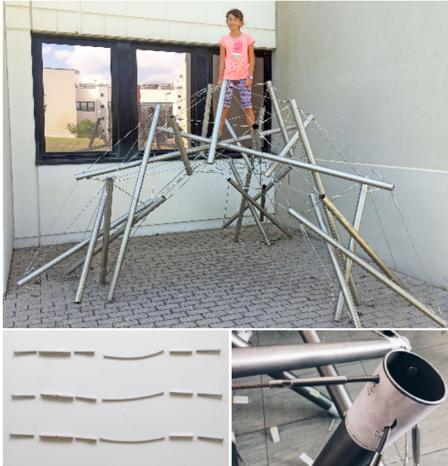
Fig. 14. Top: The rigidity of our structures allows a person to climb on them without introducing deformations. Bottom: The metallic components and labelling used for assembly.
