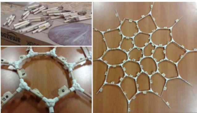
Figure 4: Hand-cut and manually labelled beams, together with a test mock-up.
