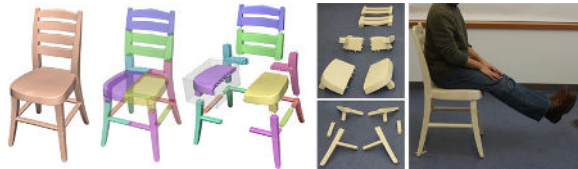
Figure 9: The Chopper approach, designed to overcome the working space limitations of current 3D printing technologies.
