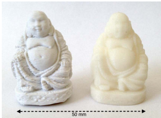
Figure 2: Two small buddhas fabricated in ABS using two different FDM machines. Given the limited size of the objects the layer structure is quite evident. Notice how the appearance properties of the material can make more or less evident both the small scale details and the printing artefacts.
