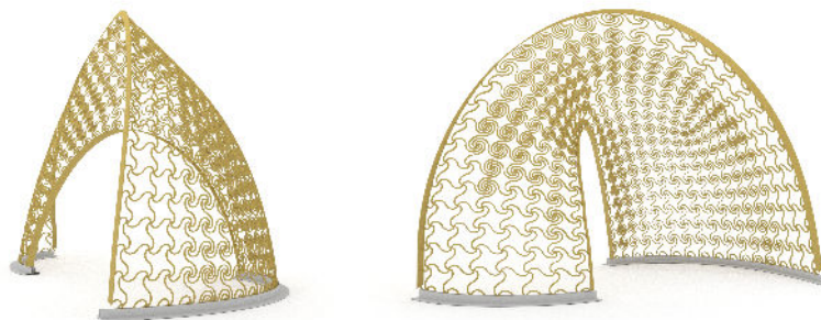
Figure 1: Overall view of the assembled plywood FlexMaps Pavilion made of bent flat panels.
