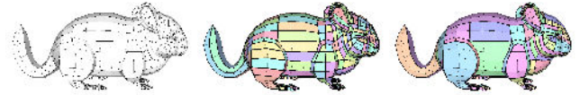
Fig. 5. On the left: the input quad layout; in the center: the patch layout with separatrices; on the right: the patch layout typical of motorcycle graph.
