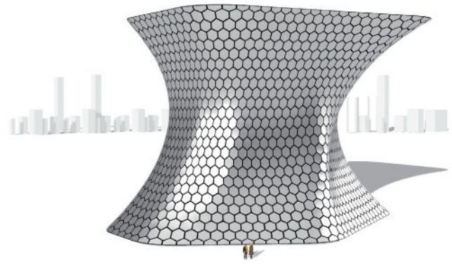
Fig. 2. A redesign of the Soumaya Museum using the proposed method. Given an initial mesh with 1,924 faces, the final group number is significantly reduced from 500 (using clustering alone) to 285 (after incorporating the proposed optimization method).
