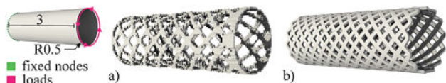
Fig. 15. (a) Cylinder beam structure obtained using topology optimization with a target volume of 0.375. The pixelated effect is caused by the voxel grid; (b) structure obtained using our method with a maximum thickness of 0.05, minimum thickness of 0.04, no support shell ( h_s = 0.00 ).
