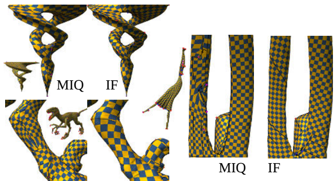
Figure 22: Three out of four models requiring cone insertion. The original result is on the left of each. On the right, the results for more isometric (but less aligned) fields generated using [Myles and Zorin 2012], for which no cone insertion was needed.
