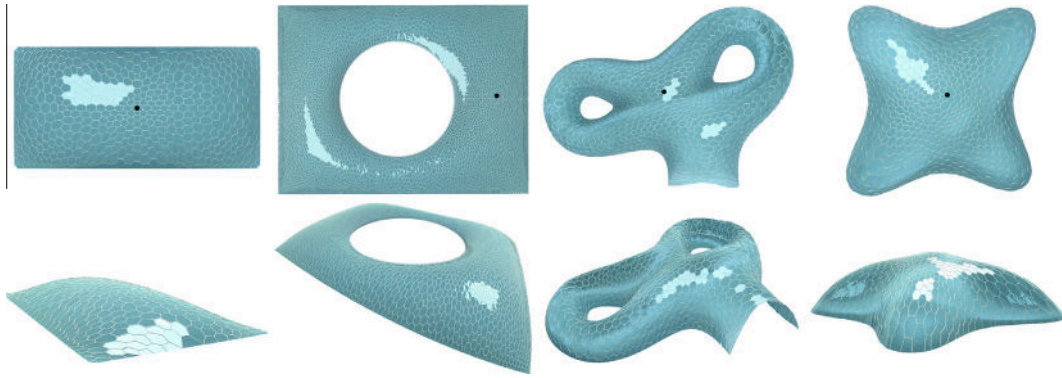
Fig. 1. All datasets. From left to right respectively: Neumünster Abbey glass roof, British Museum great court glass roof, Aquadom and Liliun Tower architectural free form shapes. The black bullet is the state parameter adopted in the geometrically non-linear analyses.
