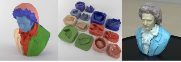
Figure 8: Nakashima et al. [NAI*18] propose an interactive method for the generation of two-piece molds for thin-shell objects. The decomposition shown on the left is generated by the solver, integrating user defined constraints (left). The method then generates a two-piece mold for each part (middle). Finally, the parts can be assembled together to form the target shape (right).
