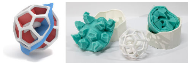
Figure 13: Alderighi et al. [AMG*19] propose an algorithm for the automatic generation of flexible, composite molds, in which the soft silicone part is supported by a hard plastic shell. The approach is based on a volumetric analysis of the mold surrounding the object to automatically generate the set of cuts needed to safely extract the cast object. On the left, the cut layout is composed of a set of internal cuts (red surfaces) and a parting surface (blue surface) separating the mold in the two pieces. On the right, the generated mold with one of the pieces opened to highlight the cut layout.
