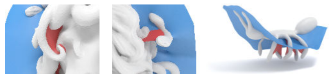
Fig. 16. Left and center: close-ups of the additional membranes on the protruding features of the Medusa head model. Right: parting surface and additional membranes on an ant model.
